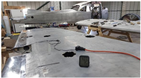
Paint stripped and installation of the STOL modifications
